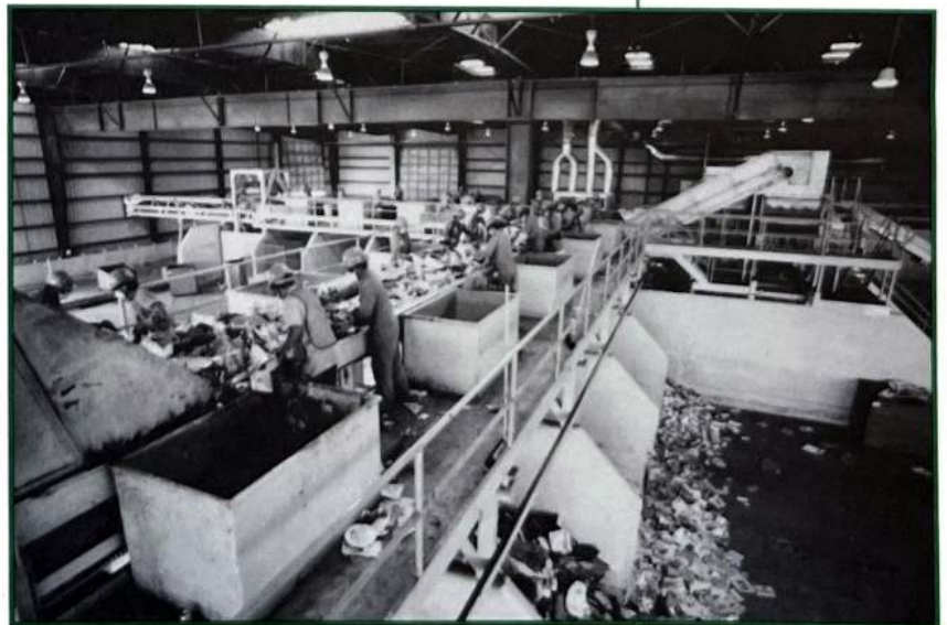
After recyclables are collected from your curbside containers, they are sent to the CVT Material Recovery Facility (MRF) for processing. This facility processes more than 3,200 tons of waste and recyclables each day!
